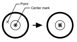
6. Completely Leveling the Instrument
