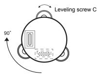
3 Repeat the procedures *1* and *2* for each 90° (100gon) rotation of the instrument and check whether the bubble is correctly centered for all four points.
