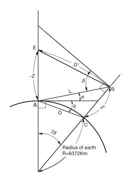
The conversion formula for horizontal and vertical distances is as follows when correction for refraction and earth curvature is not applied. D=L•cosα Z=L•sinα
