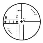
3)Shift the vertical cross-hair line and coincide it with Point D, by revolving the left and right capstan adjustment screws with the adjusting pin.Upon completing the adjustment, repeat the checking operation once more.
