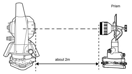
2) Sight through the eyepiece and focus to the prism. Then center the prism on the cross hairs.
