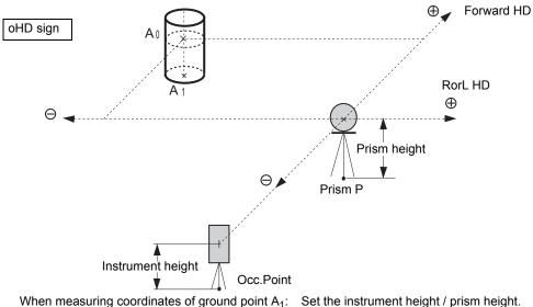
When measuring coordinates of ground point  $A_1$ : When measuring coordinates of point  $A_0$ :
