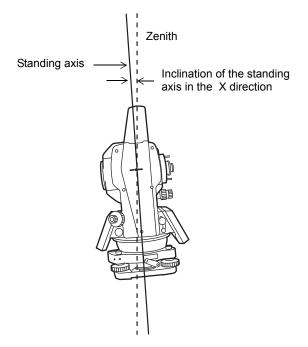
CYGNUS compensates the vertical angle reading due to inclination of the standing axis in the X directions.
