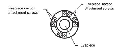
2) Loosen all four attachment screws slightly with the accessory screw-drive (while taking note of the number of revolutions).
